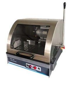
Suitable for cutting all kinds of specimens including metallic materials and nonmetallic materials to observe metallographic structure and lithofacies structure.
